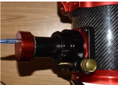
Figure 8 Example of Ocal Collimator fitted to a Newtonian Telescope
