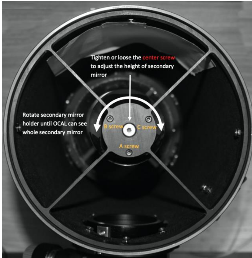
Figure 13 Adjusting the Secondary Mirror. On this Newtonian the length of the spider arms are fixed.
